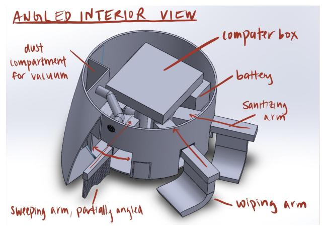
The vacuum is located under the front end of the body, opposite to the waste bin opening. The robot travels in a linear pattern (without axial rotation) across the table, covering the entire area except those covered by objects that should not be moved. This process picks up all dirt and crumbs, holding them in the dust compartment while the air runs through a filter and out the back of the robot. The compartments that contain both the garbage and dust are detachable for quick and easy disposal.
