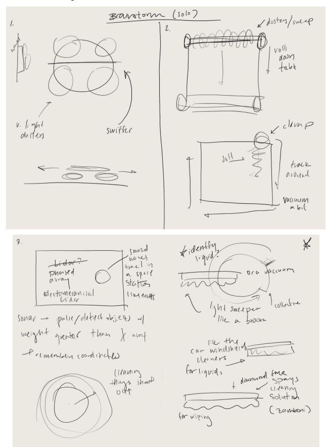
Multiple different designs were considered for the project, including ones that would clamp on the side or attach to the wall. Ultimately, it was decided that a rotating disk that descended from the ceiling would be best.
